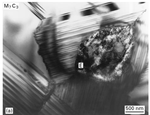
Figure 2 (a) TEM micrograph of the eutectic M_7C_3 carbides and eutectic matrix (E). Streaking contrast in carbides from defects on \{10\bar{1}0\} and \{11\bar{2}0\} planes. (b) and (c) Diffraction patterns from faulted M_7C_3 carbides. Fig. 2b showing contrast from streaking in directions of type [10\bar{1}0] and Fig. 2c showing contrast from streaking in directions of type [11\bar{2}0] .
