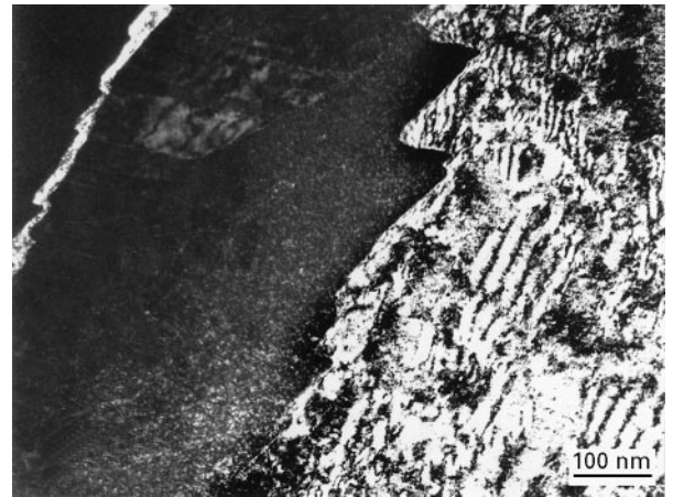
Figure 11 Dark field image of a region adjacent to a eutectic M_7C_3 carbide in the heat treated alloy. Contrast is visible from a morphology similar to that seen by Ricks et al. [25] in an Fe-Cr-Ni alloy which was identified as Widmanstätten ferrite sawteeth. In this case SAED was used to identify the illuminated phase as bcc iron.
